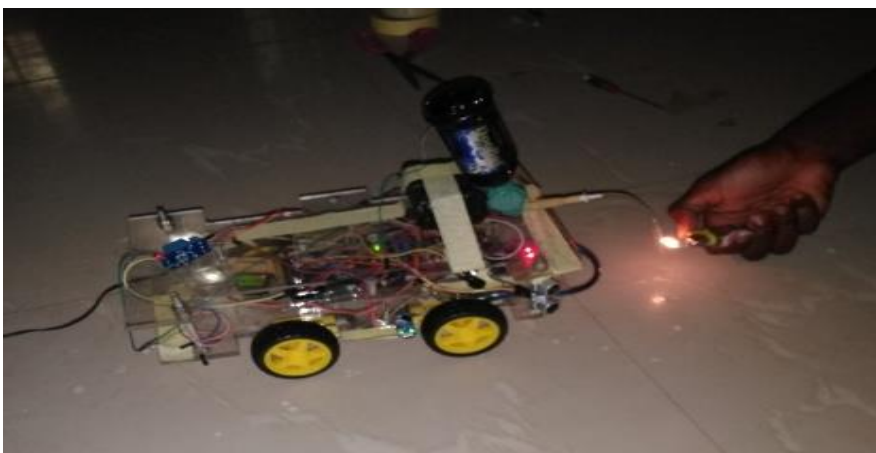
Figure 16: Robot Extinguishing Fire
