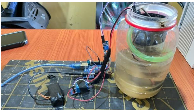
Figure 3: Prototype setup showing the automated irrigation system in dry soil condition before irrigation.
