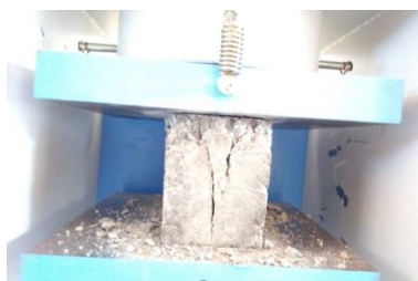
Figure 2: Indication of Compression Test
