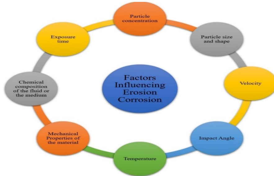
Fig. 3: Factors that affect the impingement erosion-corrosion [8]
