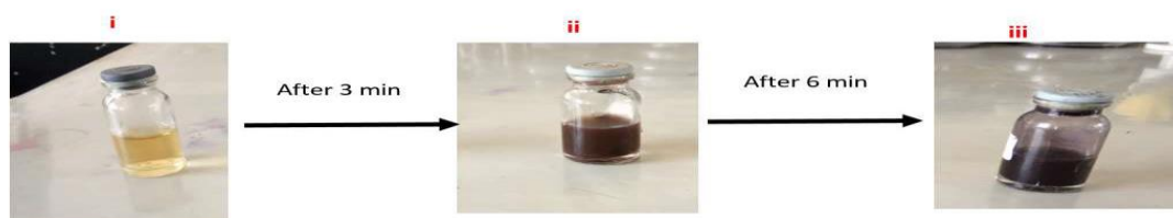
Figure 1.0: Showing the color development during the formation of gold nanoparticles by use of croton megalocarpus leaves as the reducing agent.
