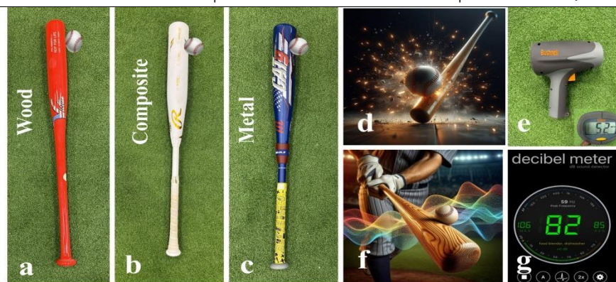
Figure 1. The bats used for experimental data collection; a) wood, b) composite, c) metal bats with their plausible interfaces with the baseball, d) Artificial intelligence (AI) generated drawing depicting the trampoline effect upon bat-ball collision, e) employed speed gun (insert shows measured speed), f) AI generated drawing demonstrating the acoustic effect using Copilot and g) screen shot of a decibel meter reading with iPhone Prox max 15.
