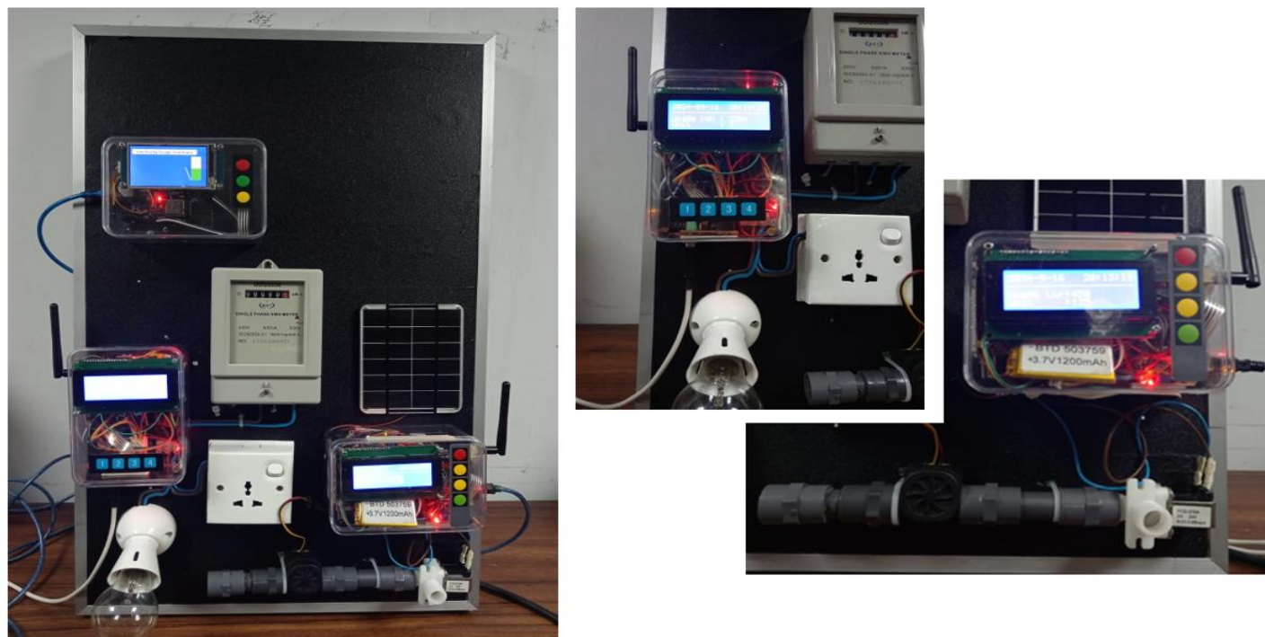
Figure 7: Smart Device for Electricity and Water Metering
