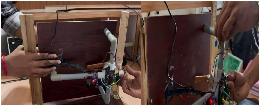
Fig 2: prototype of patternized secret knock detecting door lock & working demonstration
