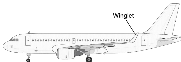
Figure 2. Schematic representation of the narrow-body A320-style aircraft used in the CFD model, emphasizing the winglet position relevant to this study's aerodynamic analysis.
