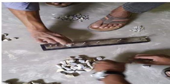
Figure 2.16: Determining a sample's length by a length gauge
