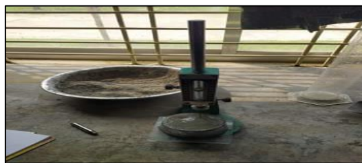
Figure 2.17: Determining normal consistency of cement by using vicat's apparatus
