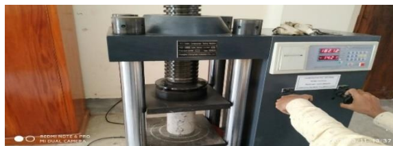
Figure 2.21: Determining the compressive strength of a cylinder using compressive load machine
