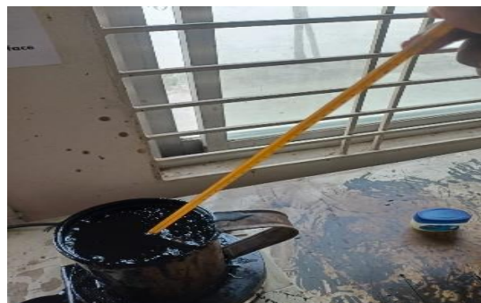
Figure 7: Heating of Bitumen till its melting point.
