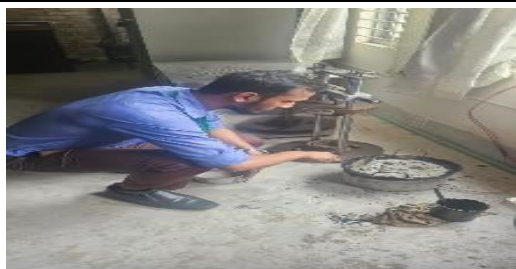
Figure 8: Mixing of CA, FA and Filler respectively and heating them on Electric Stove
