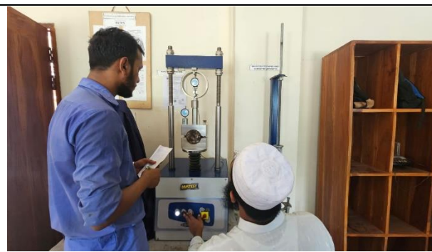
Figure 13: Putting the Specimen inside Marshall Testing Machine to obtain values
