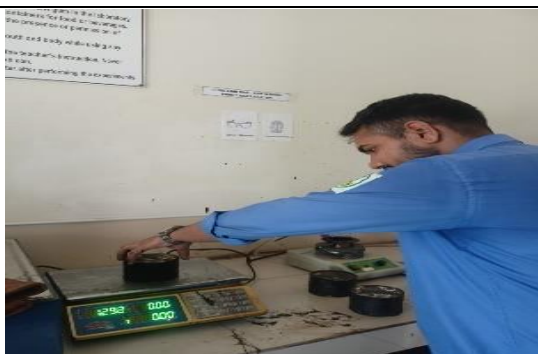
Figure 12: Taking SSD Weight after 30 minutes of water bath at 60°C
