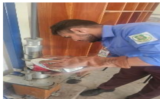
Figure 10: Adding the bituminous mix into the compaction machine and compacting to make a specimen
