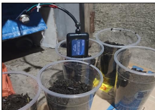
Figure 2 Individual Compost Parameters Reading Using the Soil Integrated Sensor
