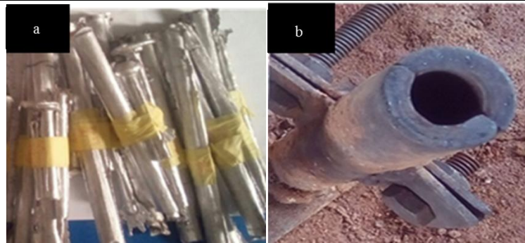
Figure 1. (a) As-cast Al-Mg-Si/GNSA composites, (b) Fabricated permanent mould [24, 26]
