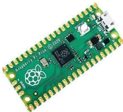
Fig 2.3: Raspberry pi pico use official power supply if possible to avoid under voltage.
