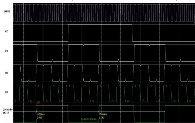
Fig. 8. Output waveform of the layout of the suggested prescaler.
