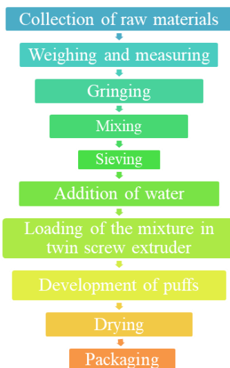
Figure 2.1 Development of Millet Puffs using Twin Screw Extruder
