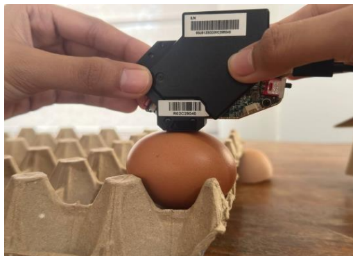
Fig. 2 Capturing of Spectral data using a portable NIR Spectrometer (horizontal position)
