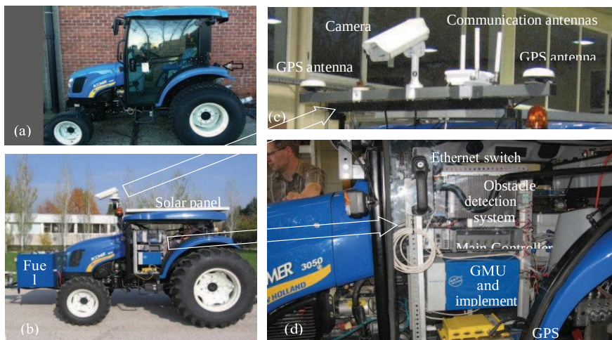
Figure 3: Description of RHEA Mobile Unit Modifications (a) Initial commercial tractor. (b) Final RHEA mobile unit after modifications. (c) External equipment mounted on the mobile unit. (d) Internal equipment distribution inside the mobile unit's cabin
