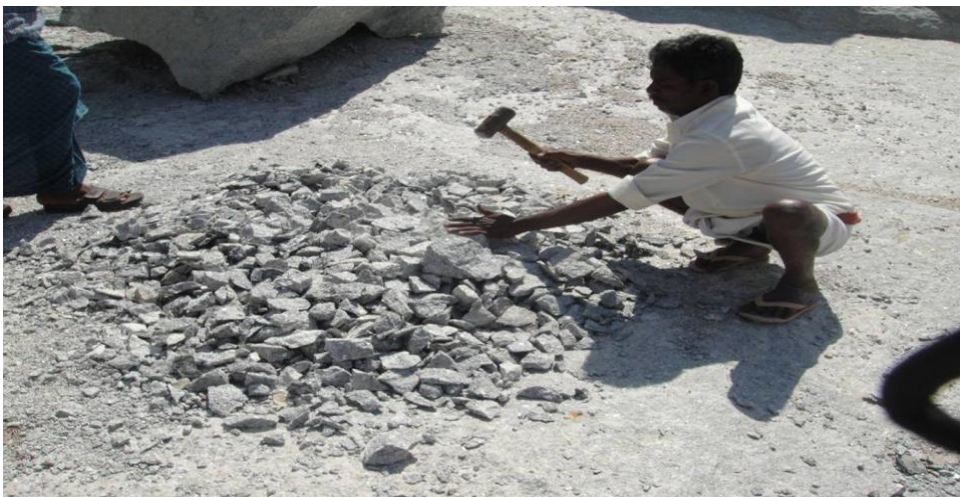
Fig. 5: Obtaining dimension stones of various sizes
