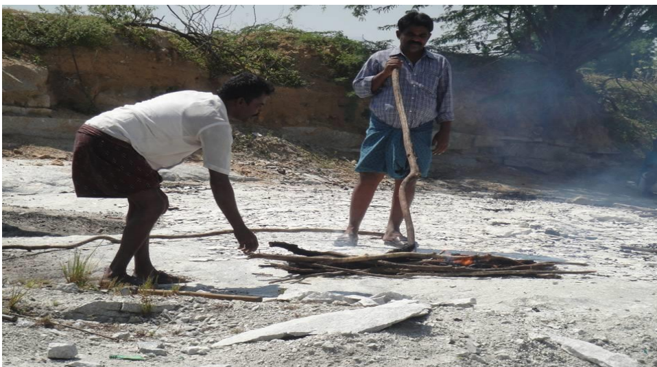
Fig. 2: Firesetting on granite of Peruru Banda
