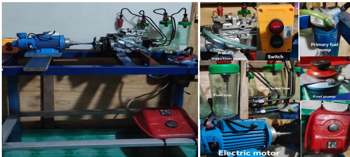
Figure 4. The diesel rotary injection pump mock-up and its components
