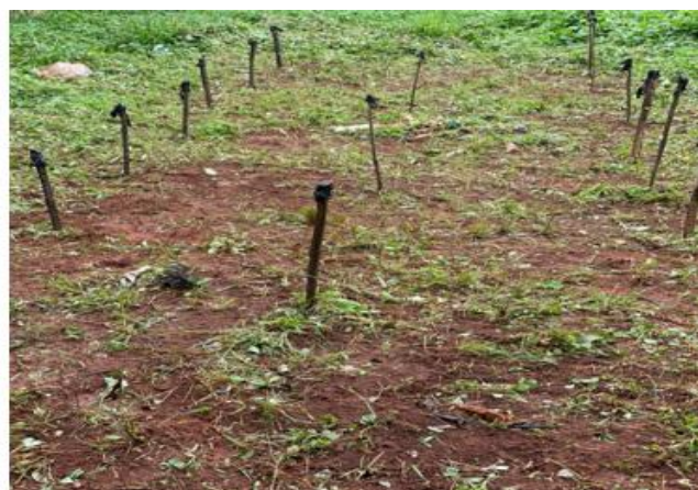
Figure 2.3: Graveyard test for treated bamboo splints
