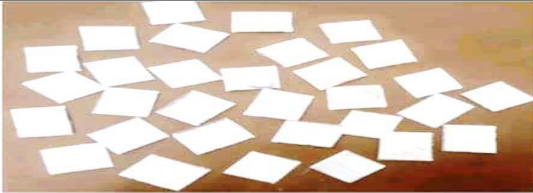
Plate 1: Top view of a sample of the sawn-out coupons from the Al 6061-alloy sheet
