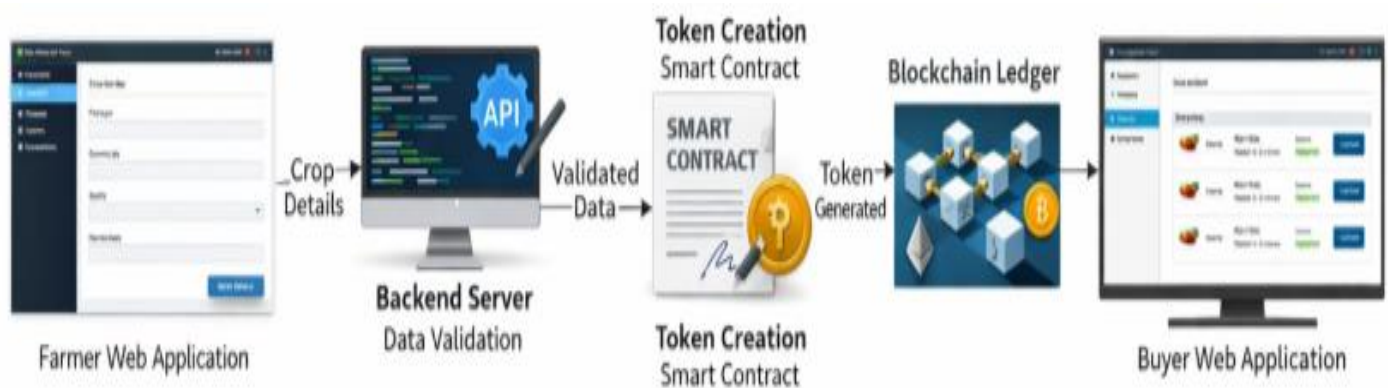
Fig 2: Implemented Tokenization Process in the Proposed Blockchain-Based Agricultural System
