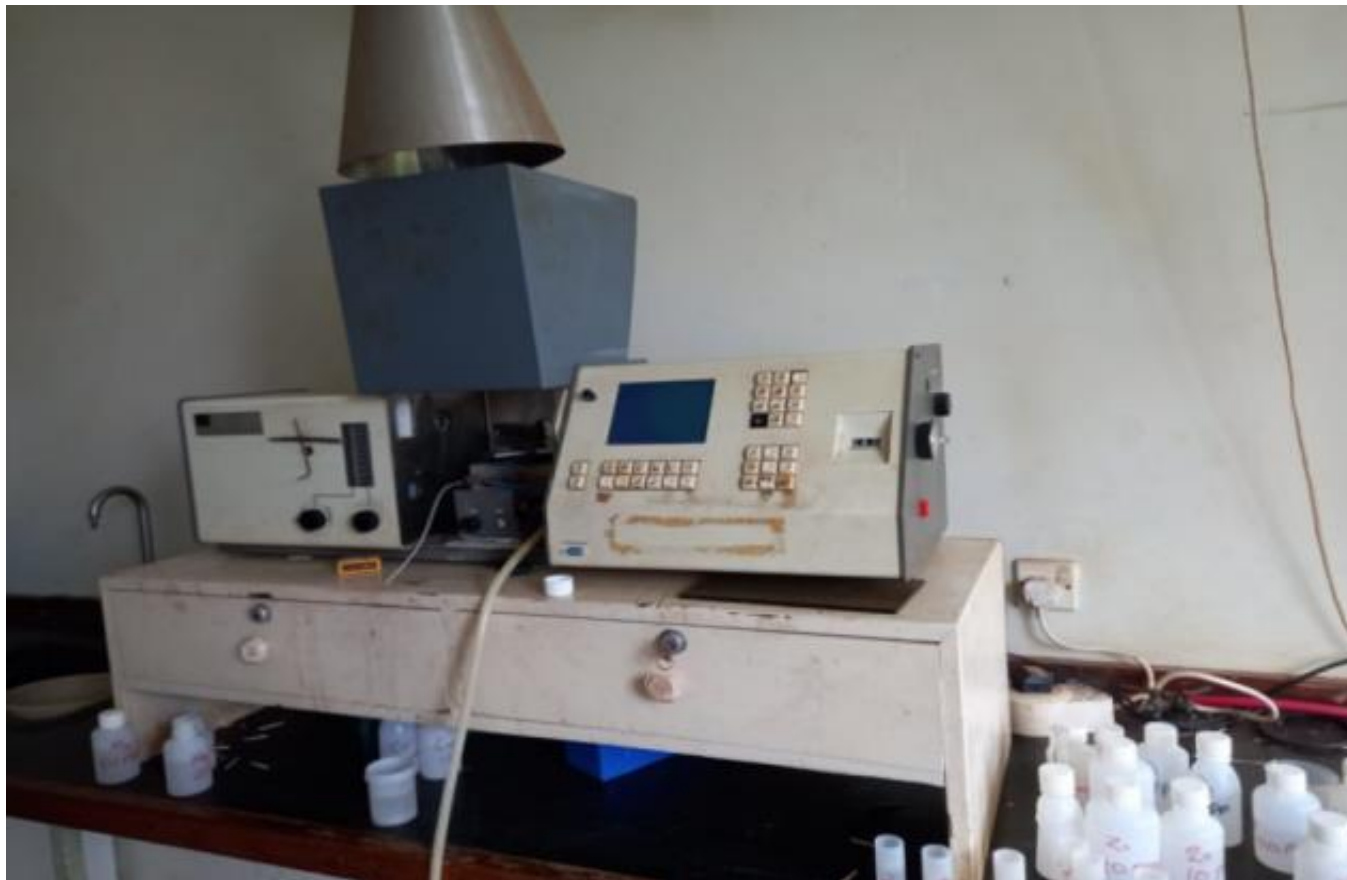
Figure 3: Atomic Absorption Spectrometry instrument used for analysis.
