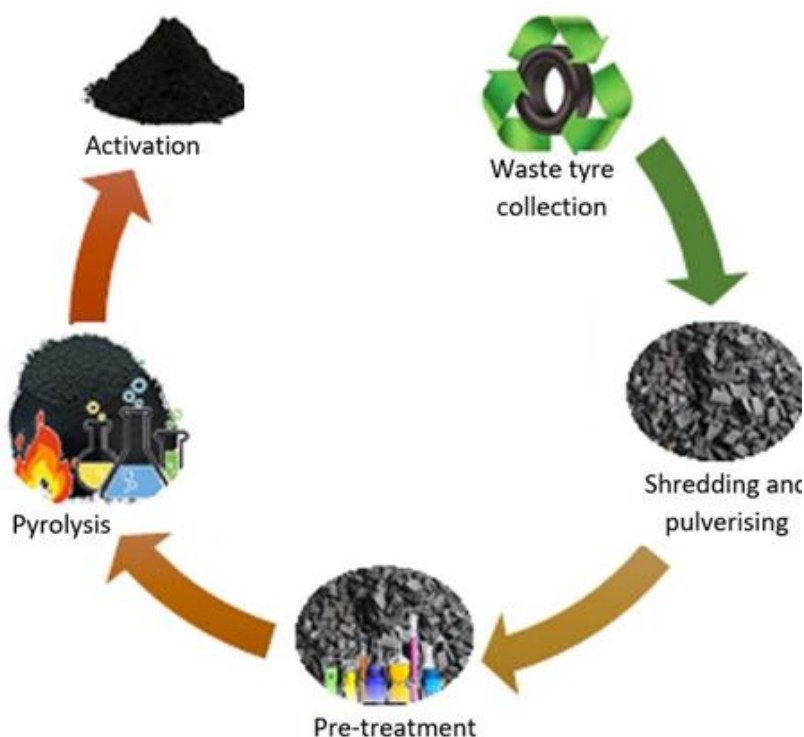
Figure 2: Process of Transforming waste tyre into Activated Charcoal
