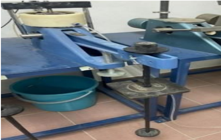
Figure 4. Setup of modified oedometer test
