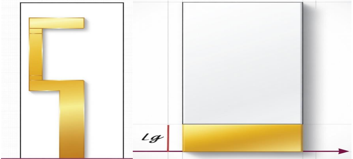
Fig 3: (a) Front view of the antenna with slot replaced with copper annealed (b) Back view
