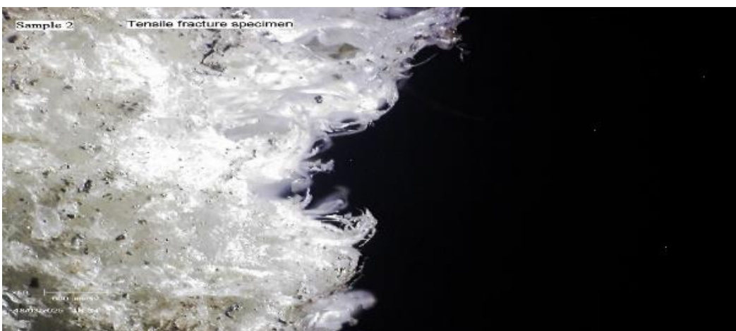
Fig.3.5: Tensile Fracture Surface Micrograph of Sample 2.
