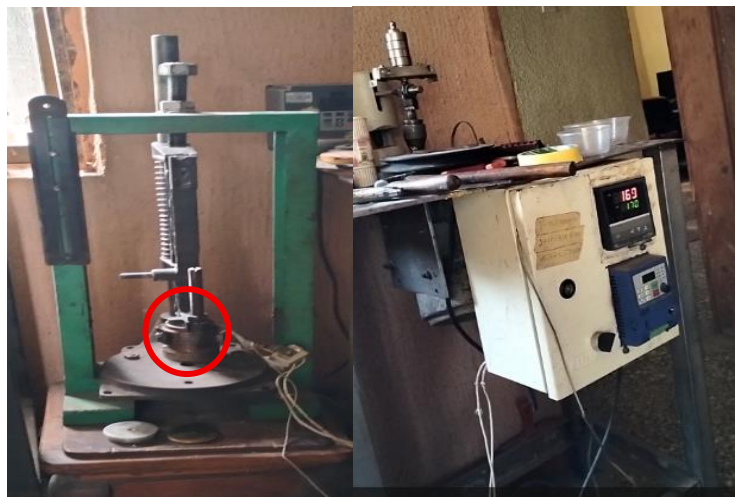
Plate 3.2b: Flat Hot Press Compression machine and Thermocouple Display Reading.
