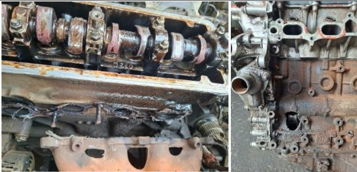
Figure 6: Engine oil leakage vs Engine block crack
