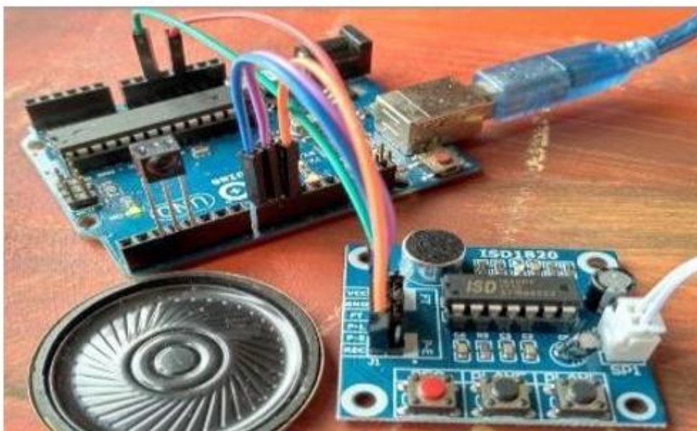
Fig. 5.2 Testing of Voice Module (ISD1820) with Speaker
