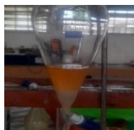
Figure 1: Biodiesel production process (a) transesterification process (b) separation process (c) produced PKO biodiesel
