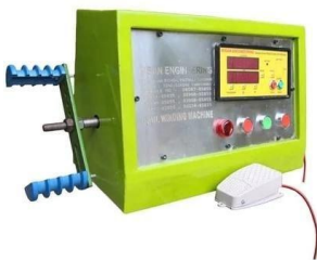
Figure 19. Digital automatic coil-winding machine used for stator rewinding.
