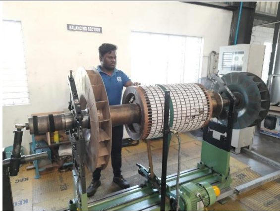
Figure 14. Dynamic balancing of a large industrial rotor assembly on a horizontal balancing machine.
