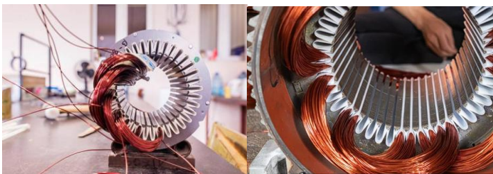
Figure 18. Winding layout comparison — double-mesh (double-layer) winding (left) and single-mesh (single-layer) winding (right).
