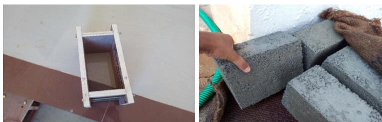
Figure 1: Mould used for preparation of specimen and specimens after Demoulding
