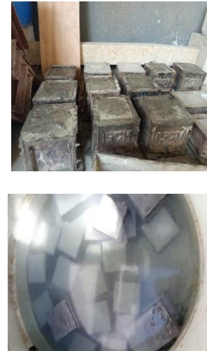
Fig 1(c): Specimen and Curing
