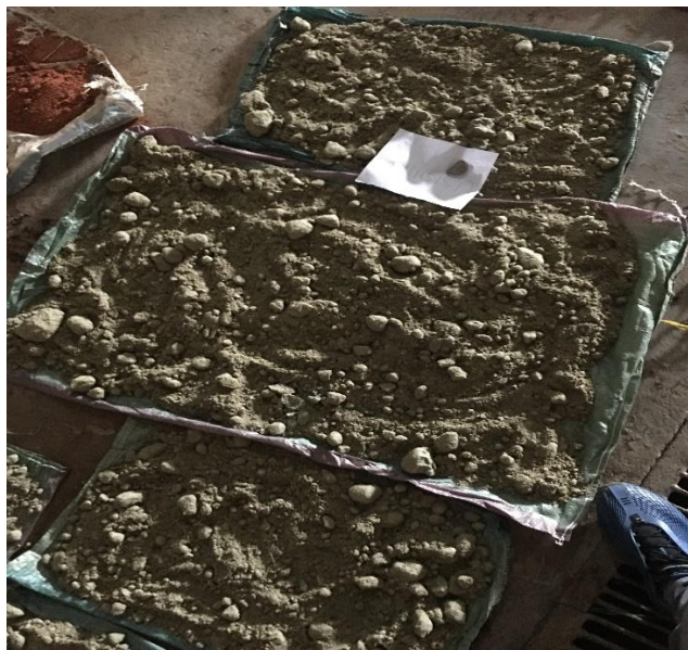
Figure 1: Gold tailings used for bricks manufacturing
